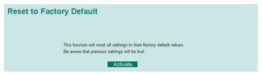
This function provides users with a quick way of restoring the TN-5500's configuration to factory defaults. This function is available in the serial, Telnet, and web consoles.
