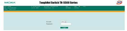
**NOTE** By default, no password is assigned to the TN-5500's web, serial, and Telnet consoles.
