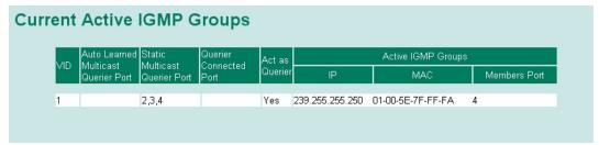
The information includes VID, Auto-learned Multicast Router Port, Static Multicast Router Port, Querier Connected Port, and the IP and MAC addresses of active IGMP groups.
